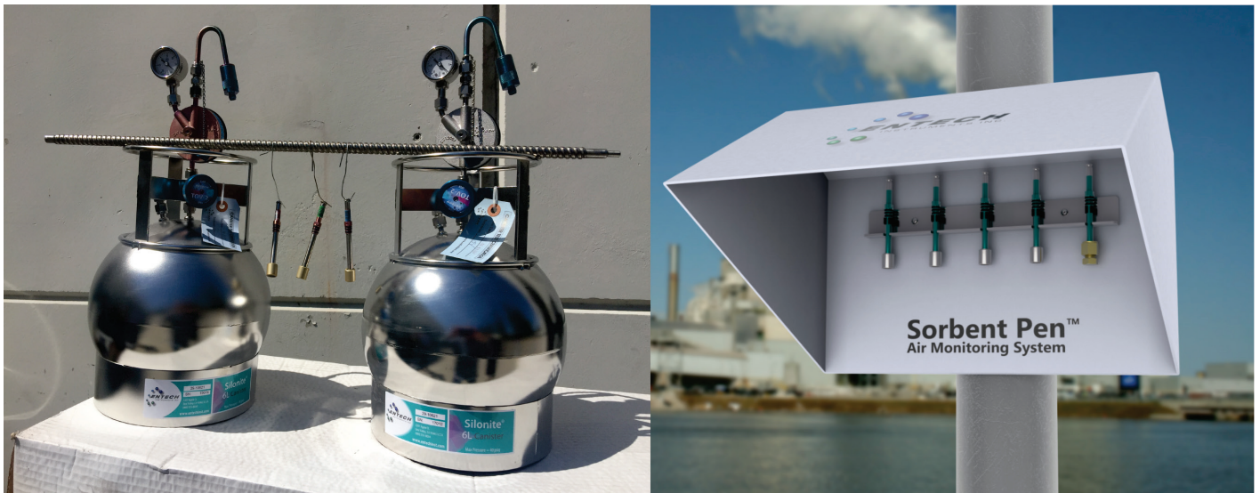
Figure 1 - One week sampling into two Silonite coated 6L canisters and 3 Diffusive Sorbent Pens with Carboxpack X. Diffuser caps are used to prevent over-sampling due to windy conditions. Also shown is a proposed sampling station for collecting multiple tubes potentially filled with different adsorbents to optimize recovery of lighter or heavier compounds.
